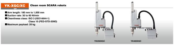
The Z-axis spline shaft is protected with bellows made of low dust emitting material and other sliding mechanisms are sealed completely. The entire harness assembly is incorporated inside the housing, and dust emission is prevented by the air suction ports located on the back of the base housing.
