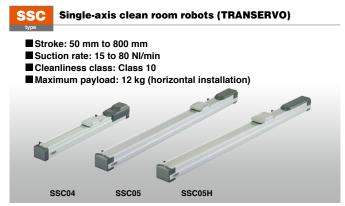
Specifications of the TRANSERVO series. TRANSERVO robots use stepper motors and a newly developed vector control system to keep performance costs low and achieve functionality similar to servomotors'. To achieve high cleanliness, these robots have suction joints installed as standard features and use grease with low dust emission. Their slide tables are also mounted with stainless steel sheets of excellent durability.
