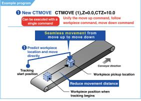
Operating conditions: YK500XG / payload 1 kg (total of workpiece and tool) / horizontal movement 250 mm / vertical movement 1 mm / conveyor speed 100 mm/sec
