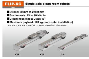
Specifications of the FLIP-X series. Whether is it a lightweight, compact model, or one with a maximum payload of 120 kg, chose one that suits your needs from the 14 available. To achieve high cleanliness, these robots have suction joints installed as standard features and use grease with low dust emission. Their slide tables are also mounted with stainless steel sheets of excellent durability.
