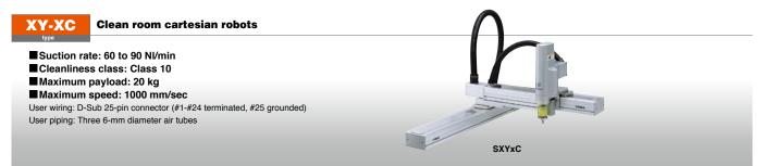
Cartesian robots for clean rooms. Using stainless steel sheets of high durability allows openings to be designed to the smallest possible, and the robots are capable of supporting Class 10 environments with minimal suction. Furthermore, with SCARA robots' high-speed units used for SXYxC robots' ZR-axis, cycle time is reduced significantly.
