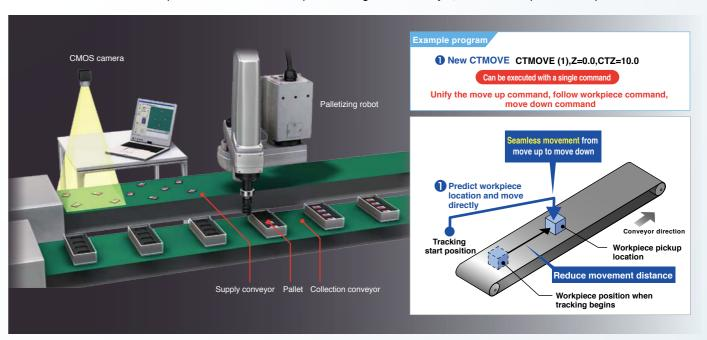
Operating conditions: YK500XG / payload 1 kg (total of workpiece and tool) / horizontal movement 250 mm / vertical movement 1 mm / conveyor speed 100 mm/sec
