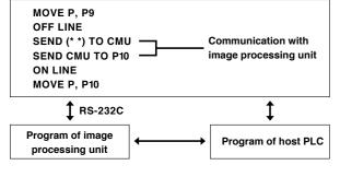
Camera and robot have separate programs
